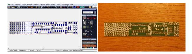
You can then send the design files to a printer circuit board (PCB) producer. The PCBs
