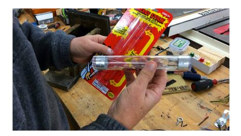
3. Attach various nuts, screws, and/or nails on each side. The more choices the harder it will be to solve. Attach one wire of the energy stick on a nail on the right side and the other to a nail on the left side. Be sure to choose a nail that conducts electricity well (like a finish nail). Attach with wire nuts (see below).
